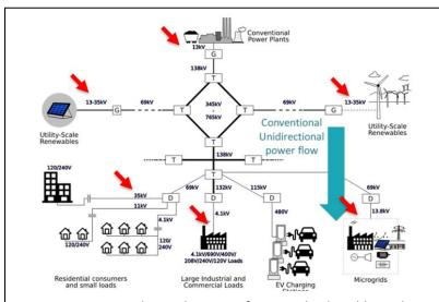
Figure 2. Diverse medium voltage interfaces need to be addressed in a modernized grid
